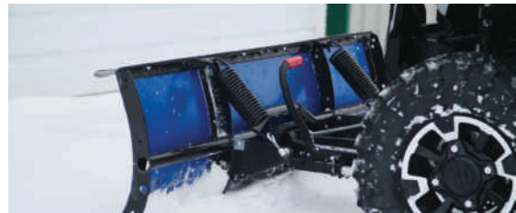
BACK DRAG MODE ALLOWS FOR PULLING SNOW AWAY FROM BUILDINGS
